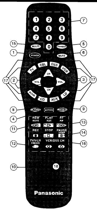
Note: In order to maximize the life of the batteries, the lights can be turned OFF and ON by pressing R-TUNE and RECALL at the same time.
